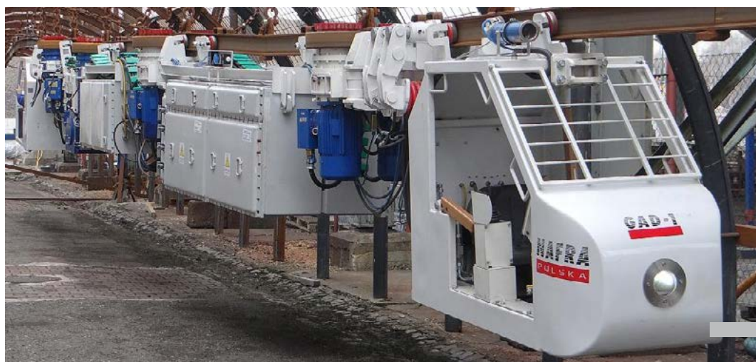
GAD-1 Battery drivetrain Implementing Company: NAFRA Polska Sp. z o.o.
