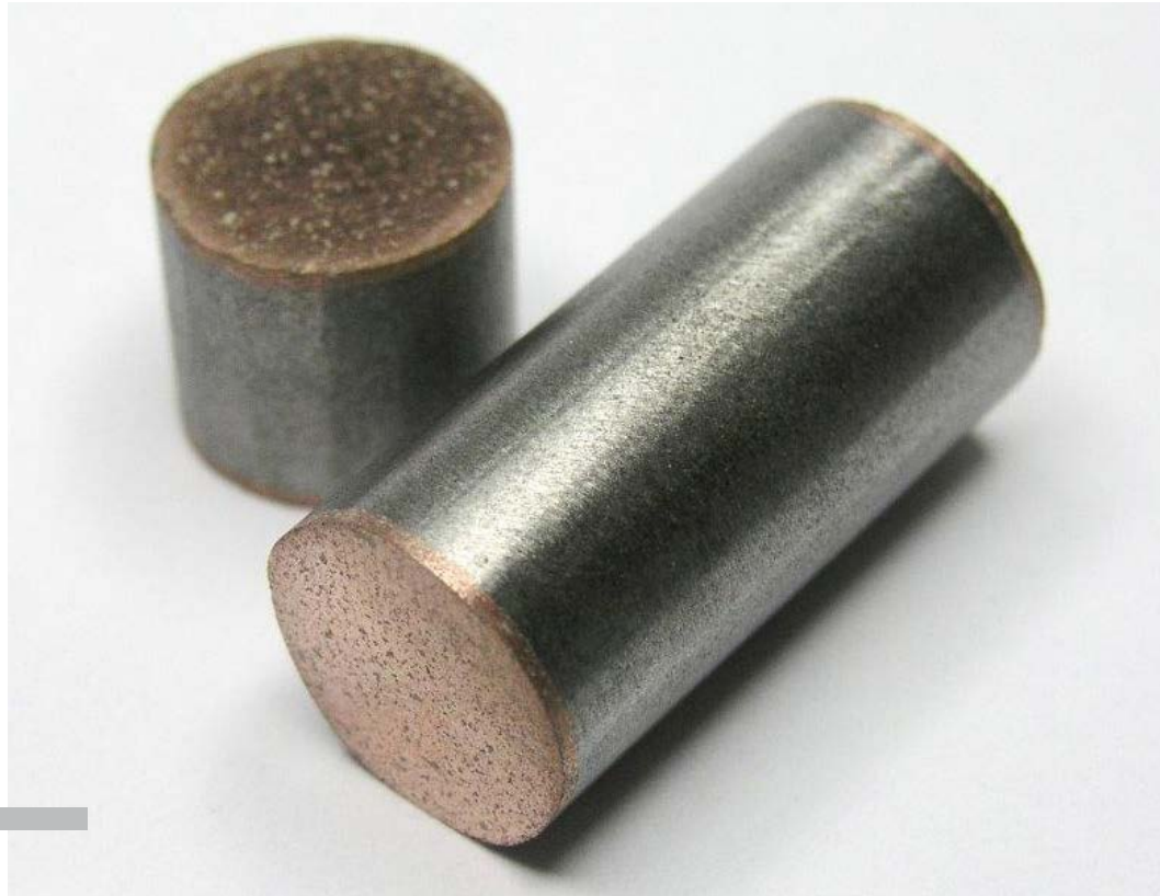
Thermoelectric semiconductor compounds with buffer cermet layer manufactured by Spark Plasma Sintering technique
