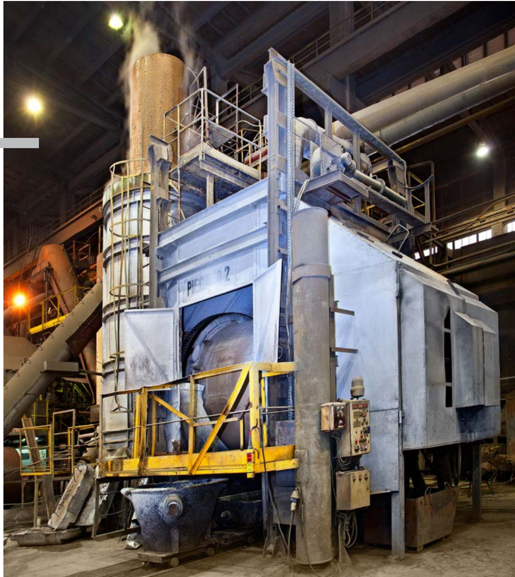
Rotary - rocking furnace for the lead alloys production
