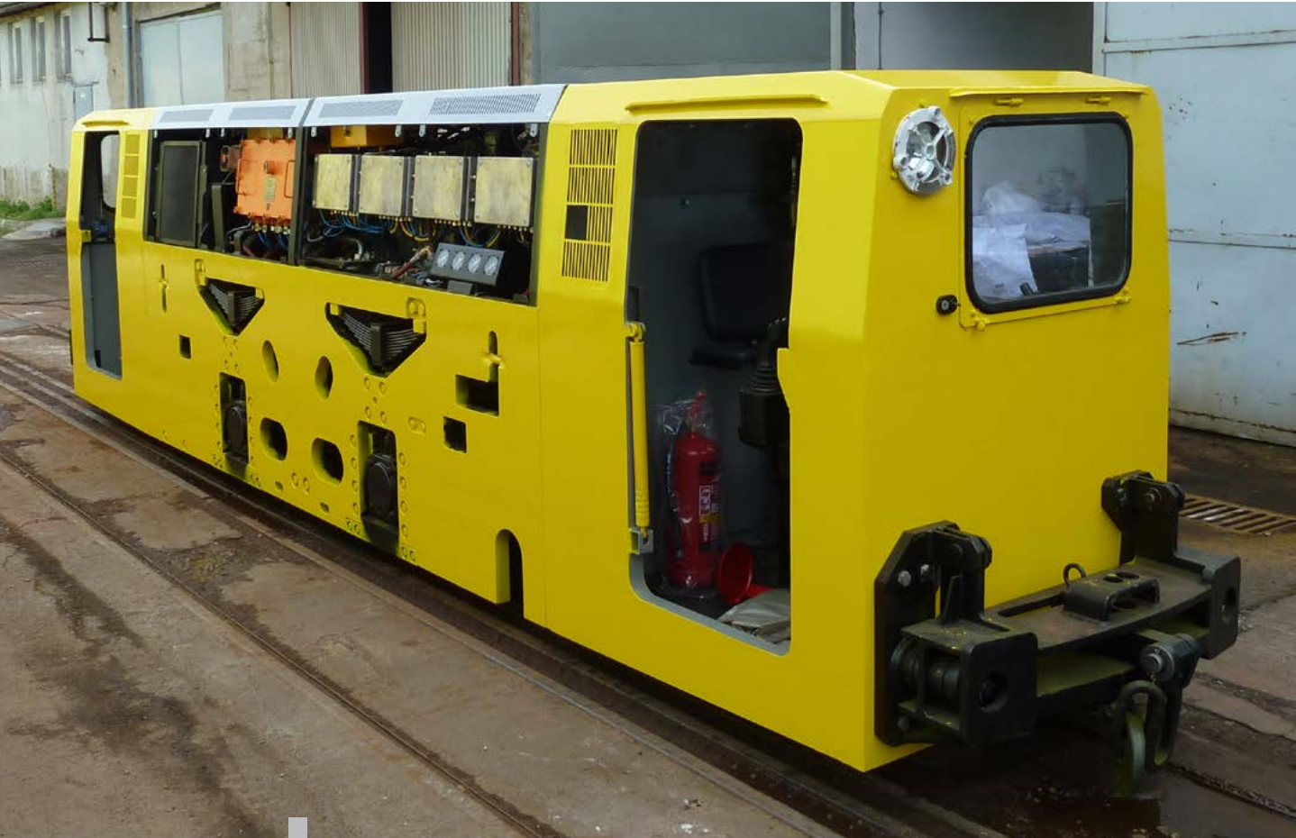
Lds-100K-EMA Under-ground diesel locomotive for mines with hydraulic transmission of torque Implementing Company: ENERGOMECHANIK Sp. z o.o.
