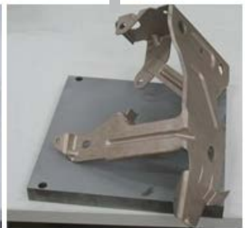
Metal elements prepared by SLS method
