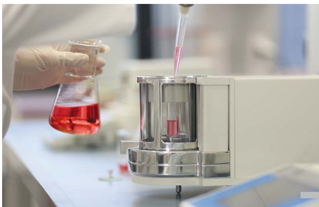
Electronic microbalance with a readability of 0.001 mg
