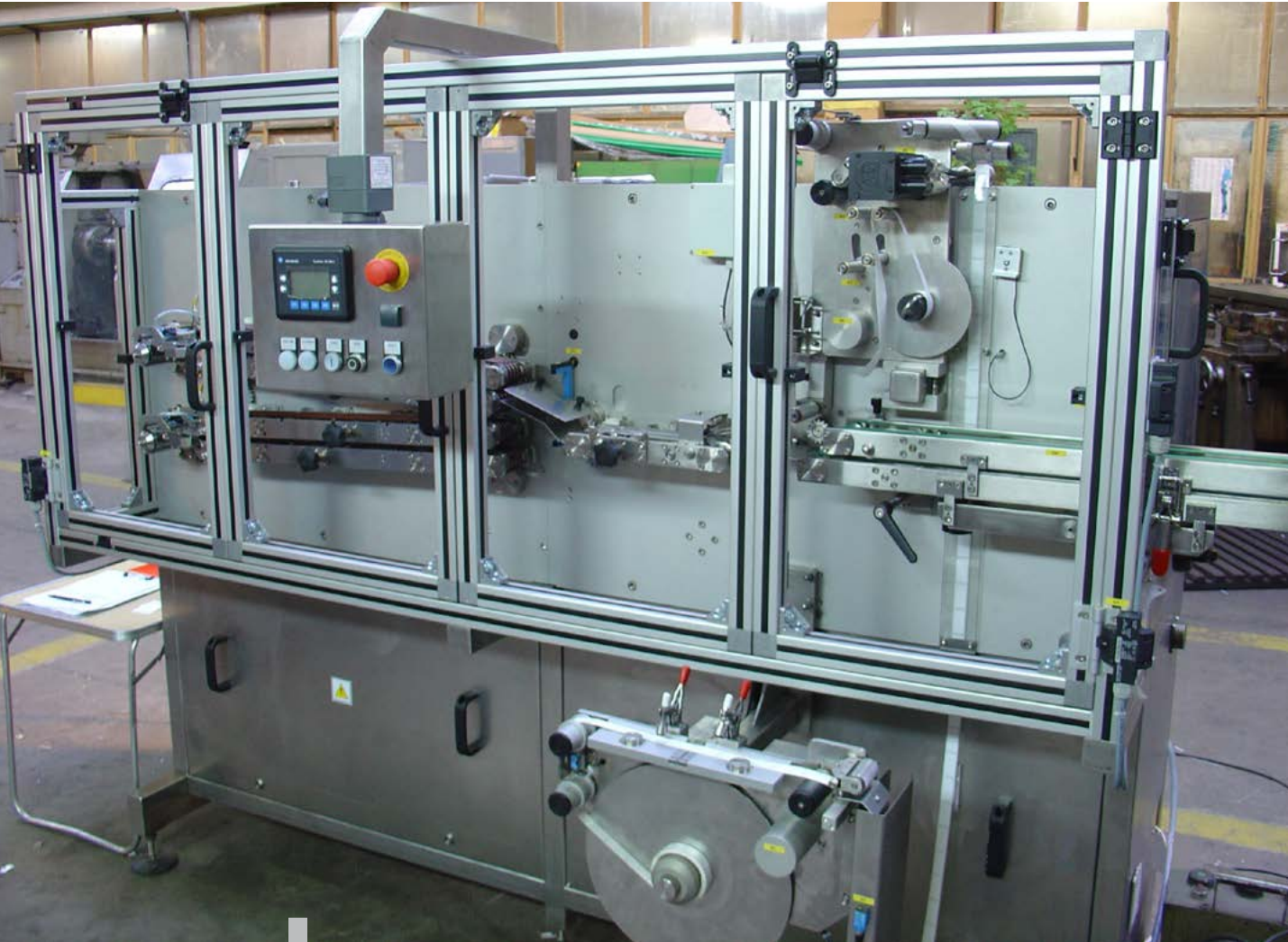
Automatic dressing strip coiling machine type AZT1
