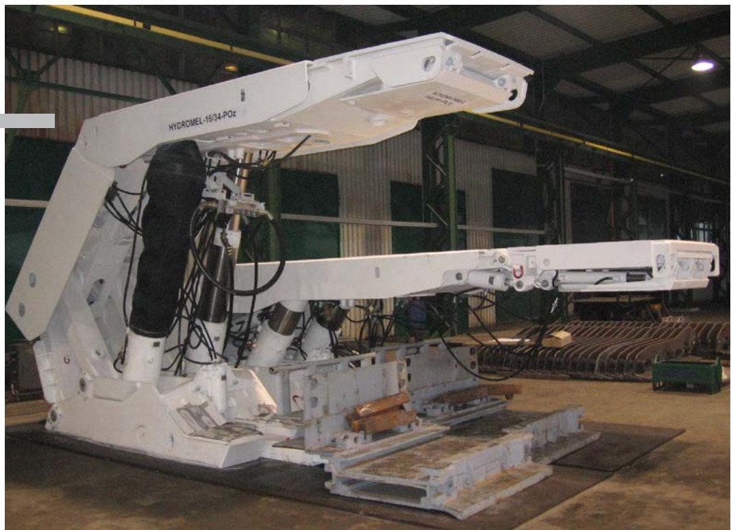
16/34 – POz Longwall Powered Roof support. Implementing Company: HYDROMEL SA
