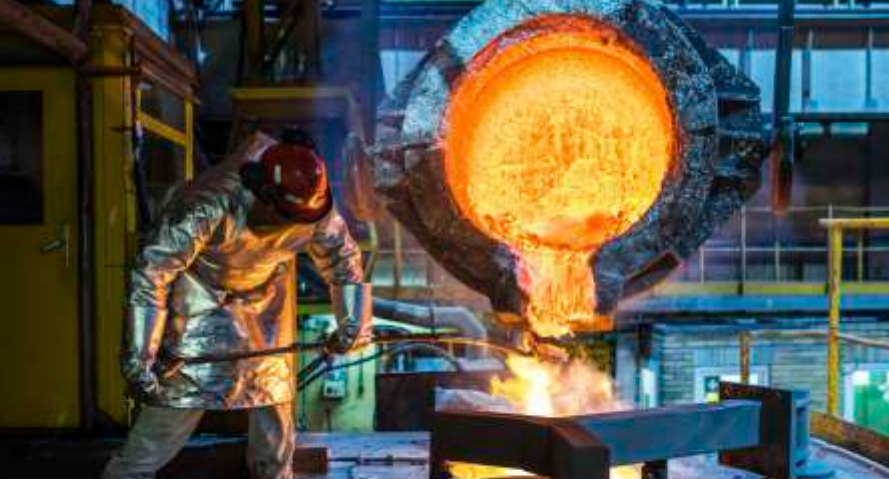
Głogów Copper Smelter/Refinery, Precious Metals Section. Charging of the anode furnace with Doré metal, containing approx. 99 % of the silver from the Kaldo furnace.
