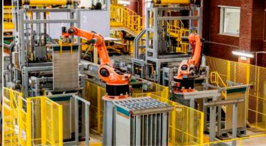
Cell House: Kuka stripping robots.
